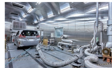
Vehicle on a chassis dynamometer in the environment simulation room
