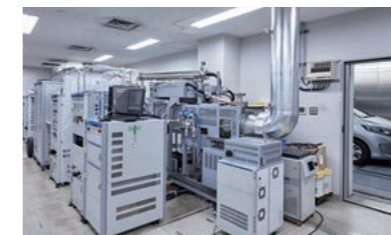
Vehicle exhaust measurement system
