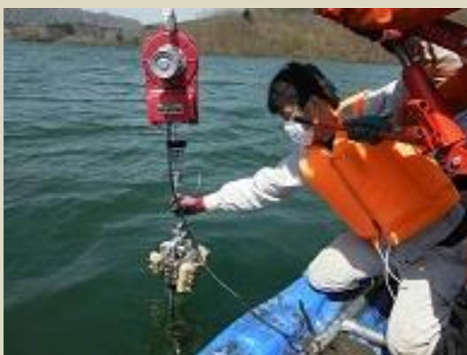
Using a sediment core sampler to collect sediment from a boat on Lake Hayama in the upper reaches of the river Manogawa in Fukushima Prefecture
