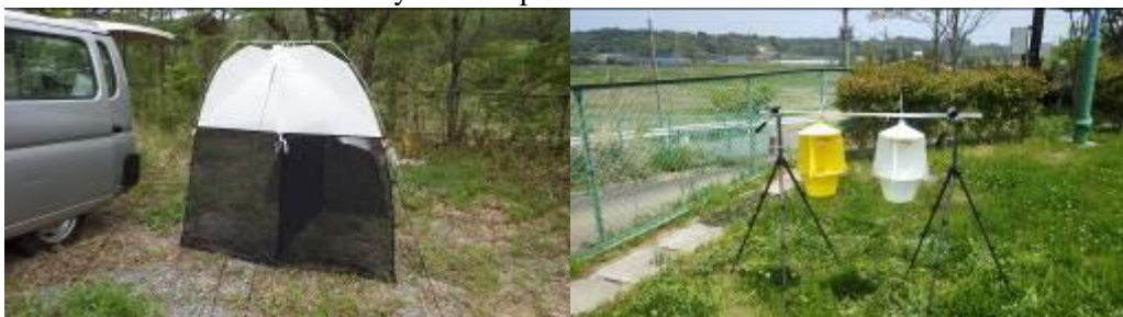
Fig. 1.3 (a) Malaise trap and (b) flight intercept trap for monitoring flying insects such as pollinators
