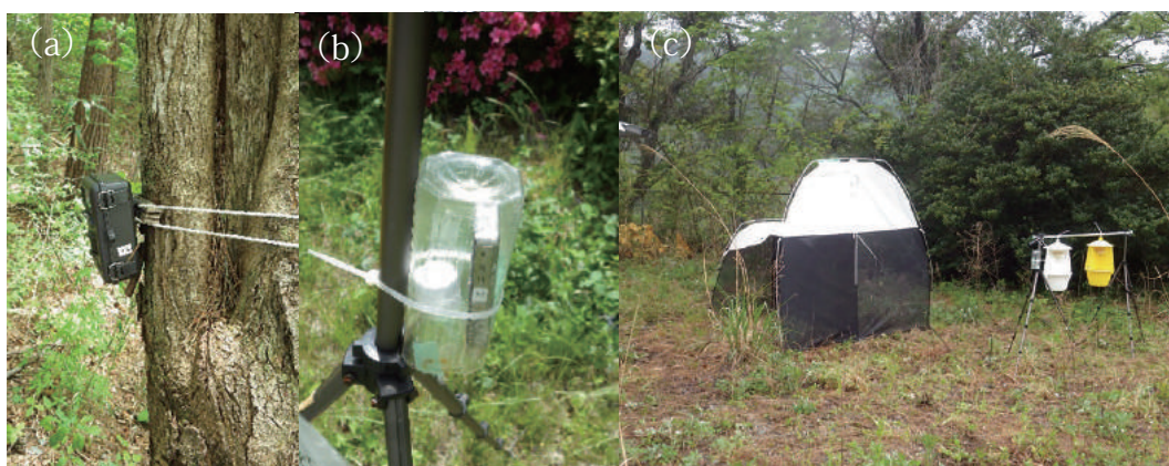
Figure 1. Equipment used for ecosystem monitoring: (a) infrared camera trap deployed in national forest etc. to monitor mammals; (b) digital recorder deployed in elementary schools etc. to monitor birds and frogs; (c) malaise trap (left) and flight interception traps (right) for monitoring insects. A digital recorder is attached to the one of the tripods supporting the flight interception traps.
