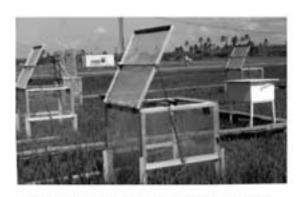
Methane emissions: field measuring system
