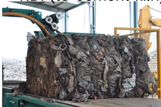
RDF (to Cement kiln)
