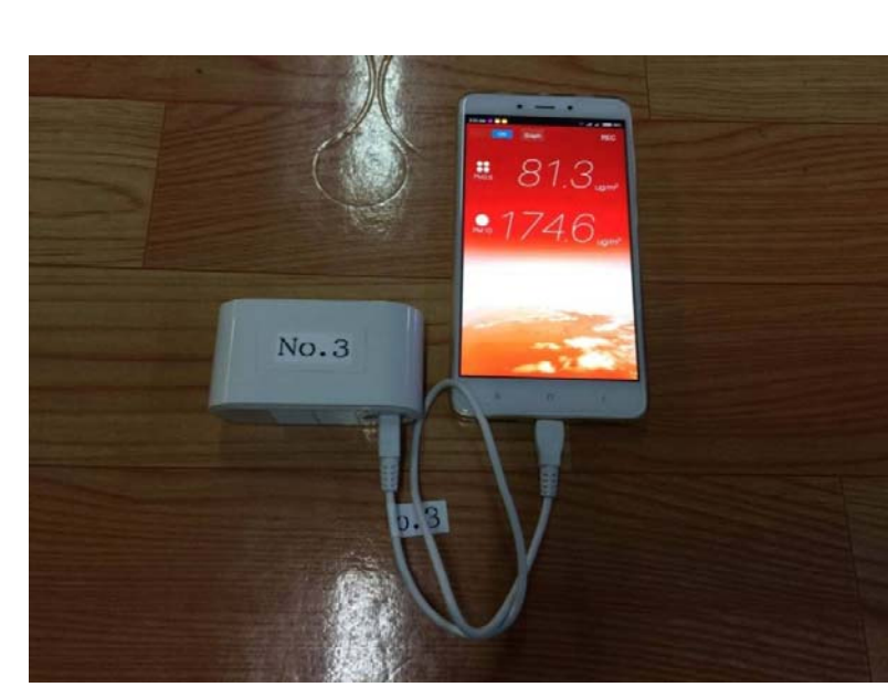
Pocket Sensor for measuring PM 2.5 and PM 10 concentration
