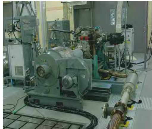
Diesel engine and dynamo for generating nanoparticles
