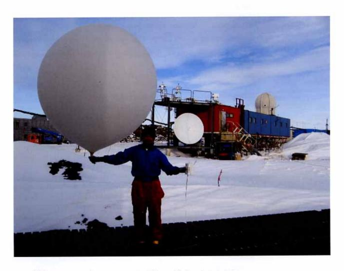
Taking ozone sonde measurements at Showa Station in Antarctica
