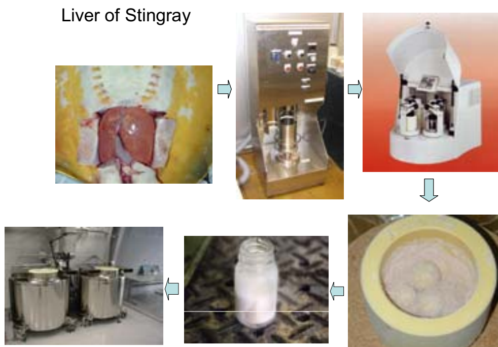
Fig. 4 Environmental Specimen Bank: stingray liver in situ after excision; coarse and fine crushing; bottling; and cryopreservation in cold \text{N}_2 vapor ( < -150\text{ }^{\circ}\text{C} ) over liquid \text{N}_2 .
