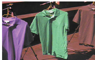
Fig. 2 Outdoor monitoring of surface temperatures of polo shirts of different colors but the same material and design during exposure to solar radiation (8 August 2011). There was an obvious inverse correlation between color brightness and measured surface temperature. For both good health and reduction of air-conditioning use, we need to choose clothing colors wisely.
