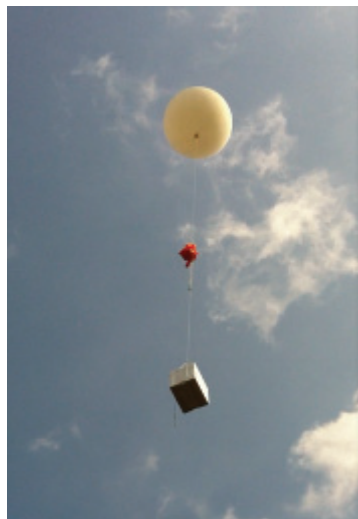
Fig. 1 The CO 2 sonde, which can reach an altituded of up to 10 km.
