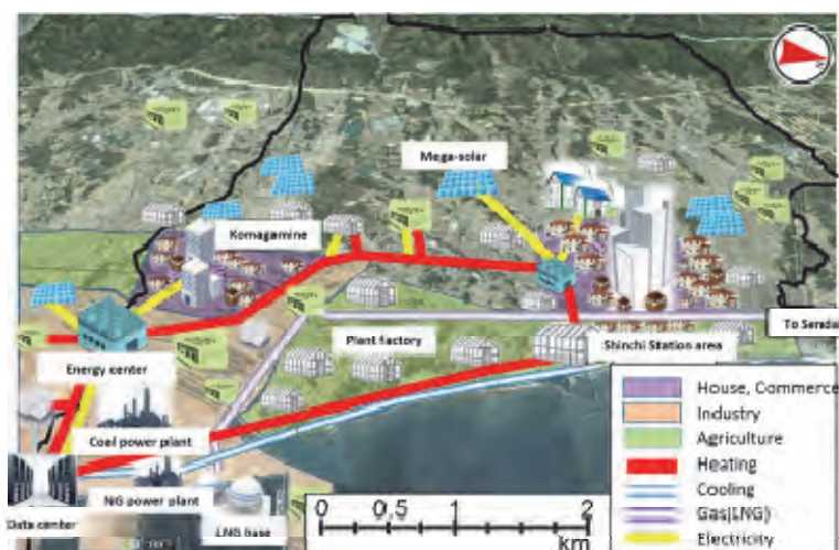
Illustration of urban revitalization planning by using regional energy, liquefied natural gas (LNG)
