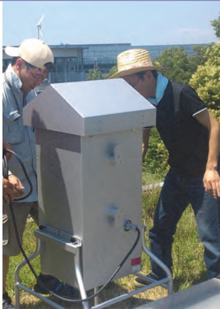
Setting up a high-volume sampler to collect particulate matter (PM) in Saitama Prefecture. Collected samples are used for toxicity studies.
