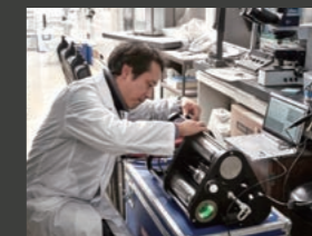
Fast repetition rate fluorometry allows us to estimate photosynthetic activity in the field.
