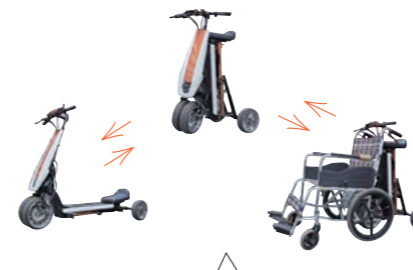
The ultra-compact personal mobility system can be transformed to suit the user type and the purpose of use (multi-purpose mobility).
