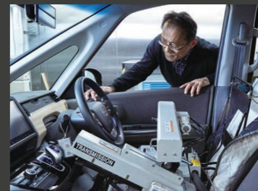
Automated driver (robot) instead of a human driver
